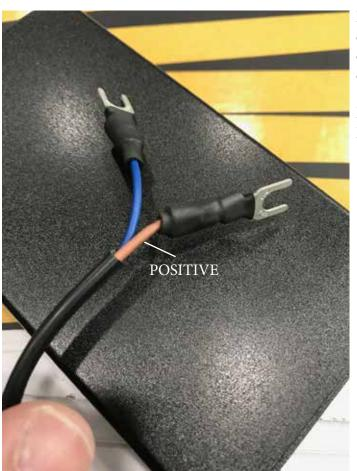
Locate the two wires coming out of the EL converter box. Note the color difference.
